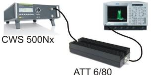
Fig 6.1 Setup for a function test
