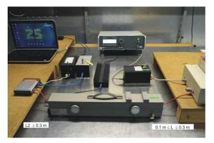
Fig 8.4 :Example Setup using EM clamp
